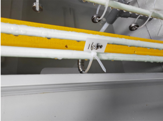
Bearings suspended in chamber (t=16:50)
