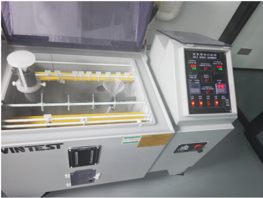
VINTEST chamber — temp 35 °C confirmed
